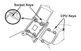
Once they are aligned, carefully lower the CPU straight down into the socket. Do not drop the CPU on the socket or move the CPU horizontally or vertically. Do not rub the CPU against the surface or against any of the socket pins to avoid damaging the CPU or the socket.
