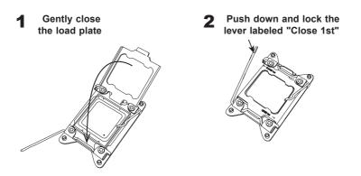
Close the load plate with the CPU inside the socket. Lock the lever labeled "Close 1st" first, then lock the lever labeled "Open 1st" second. Using your thumb, gently push the load levers down to the lever locks.
