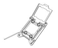
Warning: You can only install the CPU inside the socket in one direction. Make sure that it is properly inserted into the CPU socket before closing the load plate. If it doesn't close properly, do not force it as this may damage your CPU. Instead, open the load plate again to make sure that the CPU is aligned properly. 7. With the CPU inside the socket, inspect the four corners of the CPU to make sure that the CPU is properly installed.
