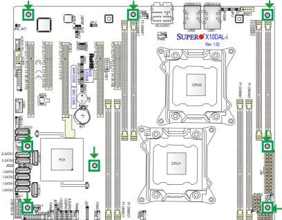
**Warning:** 1) To avoid damaging the motherboard and the components, please do not use the force greater than 8 lb/inch on each mounting screw during motherboard installation. 2) Some components are very close to the mounting holes. Please take precautionary measures to avoid damaging components when installing the motherboard to the chassis.
