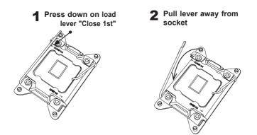
With the lever labeled "Close 1st" fully retracted, gently push down on the lever labeled "Open 1st" to open the load plate. Lift the load plate to open it completely.
