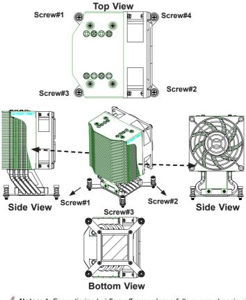
**Notes:** 1. For optimized airflow effency, please follow your chassis airflow direction to install the heatsink. 2. Graphics shown in this manual are for reference only. They may or may not look the same as the components installed in your system.
