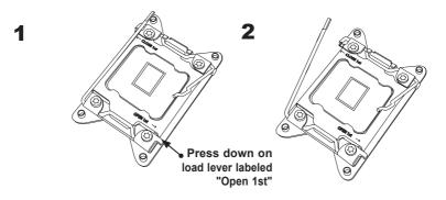
Note: All graphics, drawings, and pictures shown in this manual are for illustration only. The components that came with your machine may or may not look exactly the same as those shown in this manual. 2. Press the second load lever labeled "Close 1st" to release the load plate that covers the CPU socket from its locking position.
